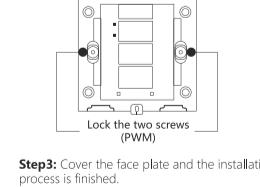
Step3: Cover the face plate and the installation process is finished.
